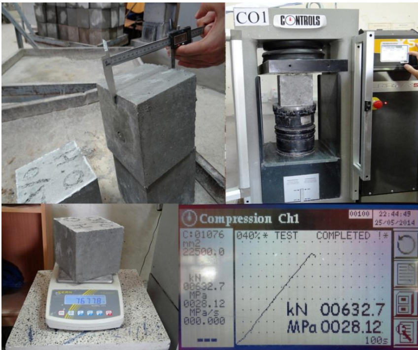
Figure-5: laboratory test (compressive strength for concrete cubes).
